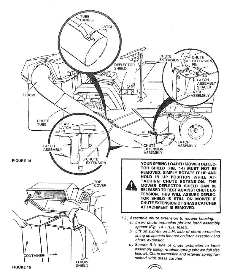
d. Secure L.H. side of chute extension to latch assembly using: latch pin and retainer spring. Retainer spring shown full size below. Latch pin and retainer spring furnished with grass catcher.
